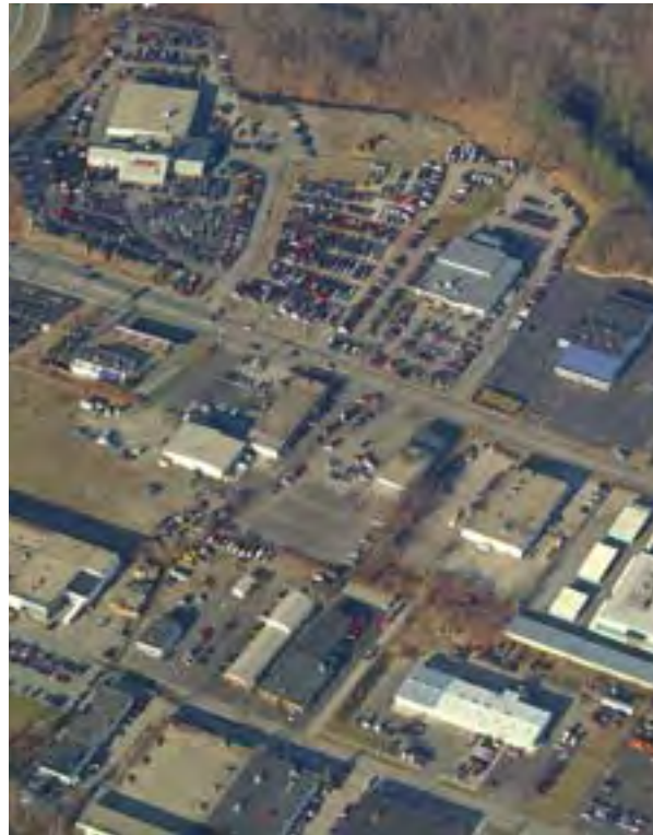
The impact of impervious cover is obvious near a typical commercial area: both the quantity and quality of runoff are impacted, and infiltration is greatly reduced.
