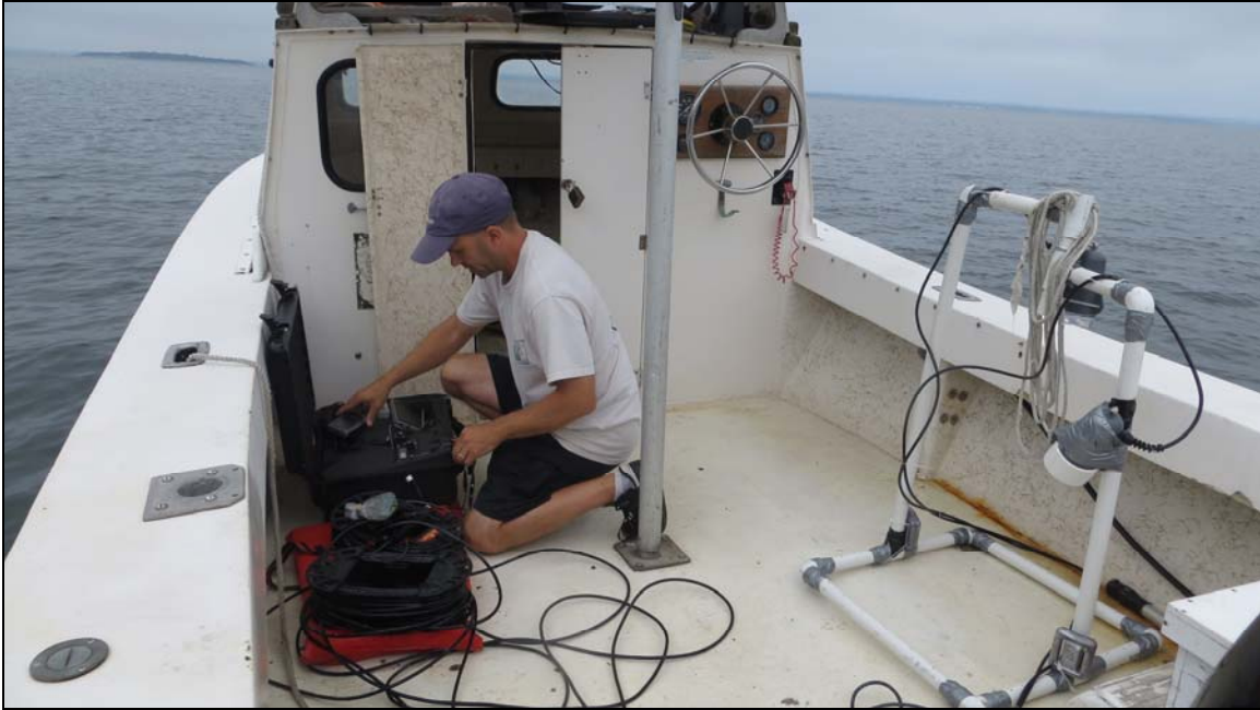
Figure 2. The tier 2 underwater video mapping system includes the camera and light, which are mounted on the PVC frame (right), and a DVR, GPS, and other accessories, which are mounted in the pelican case (left).
