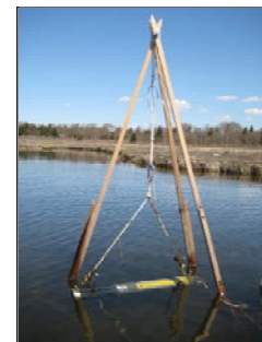
Deploying structure and sonde at Nag Creek
