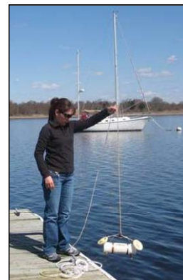
NBNERR staff collecting water with the grab sampler.
