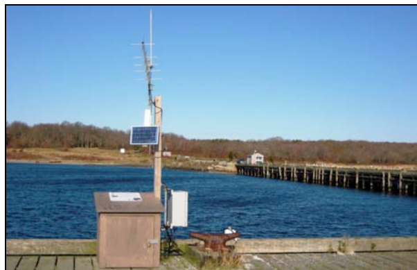
Figure 7. The telemetry station transmits water quality data from the T-Wharf Bottom station via satellite. The near-real time data collected can be accessed and downloaded online at http://cdmo.baruch.sc.edu/QueryPages/googlemap.cfm .
