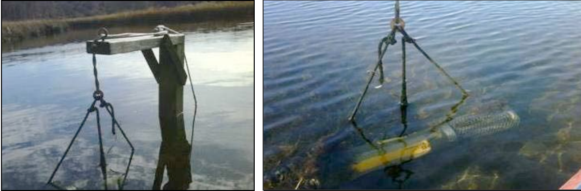
Figure 5. Deployment structure at Nag Creek (left) and the sonde in the water (right).
