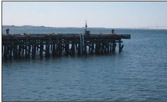
Figure 4. Two water quality monitoring stations are located at T-Wharf: Surface and Bottom (left and right PVC pipes, respectively).
