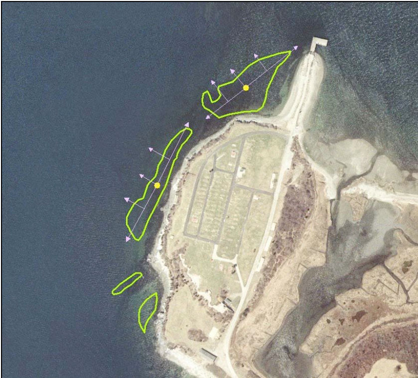
Figure 2. The basic strategy for groundtruthing eelgrass delineations is to collect video and GPS data at the middle and edges of the polygon (intersections of the arrows and the green line).
