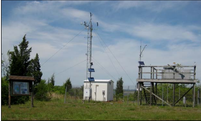
Figure 11. Picture of the meteorological station at Potter Cove showing the wooden platform and aluminum tower where the sensors are located for the collection of atmospheric data.
