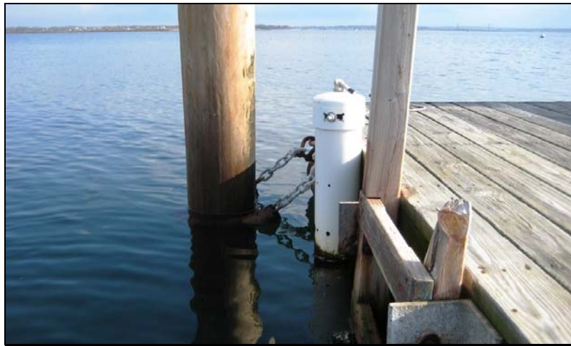
Figure 6. Picture of the current deployment structure at Potter Cove; a PVC pipe attached to a floating dock.
