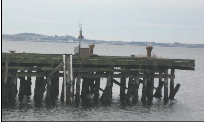
Figure 5. Two water quality monitoring stations are located at T-Wharf: Surface and Bottom (left and right PVC pipes, respectively).
