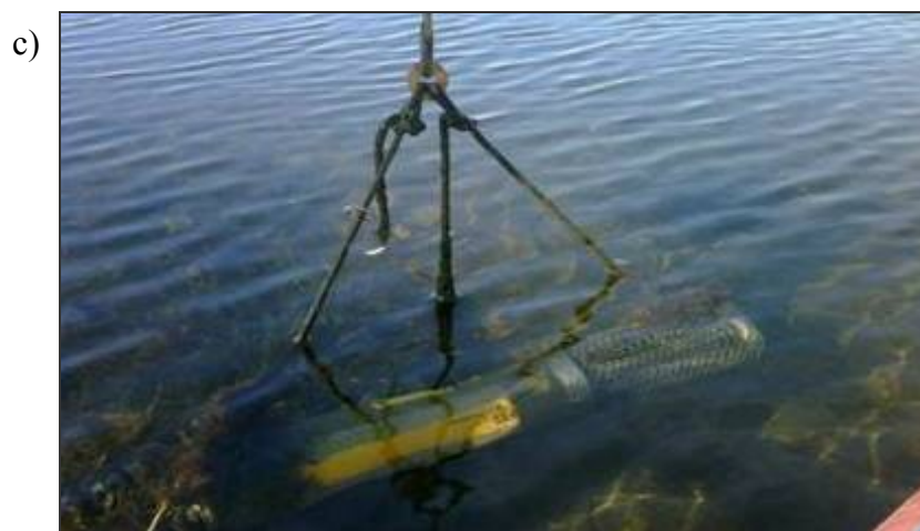
Figure 7. Deployment structure at Nag Creek: diagram of the deployment structure (a), structure in the field (b), the sonde in the water (c).
