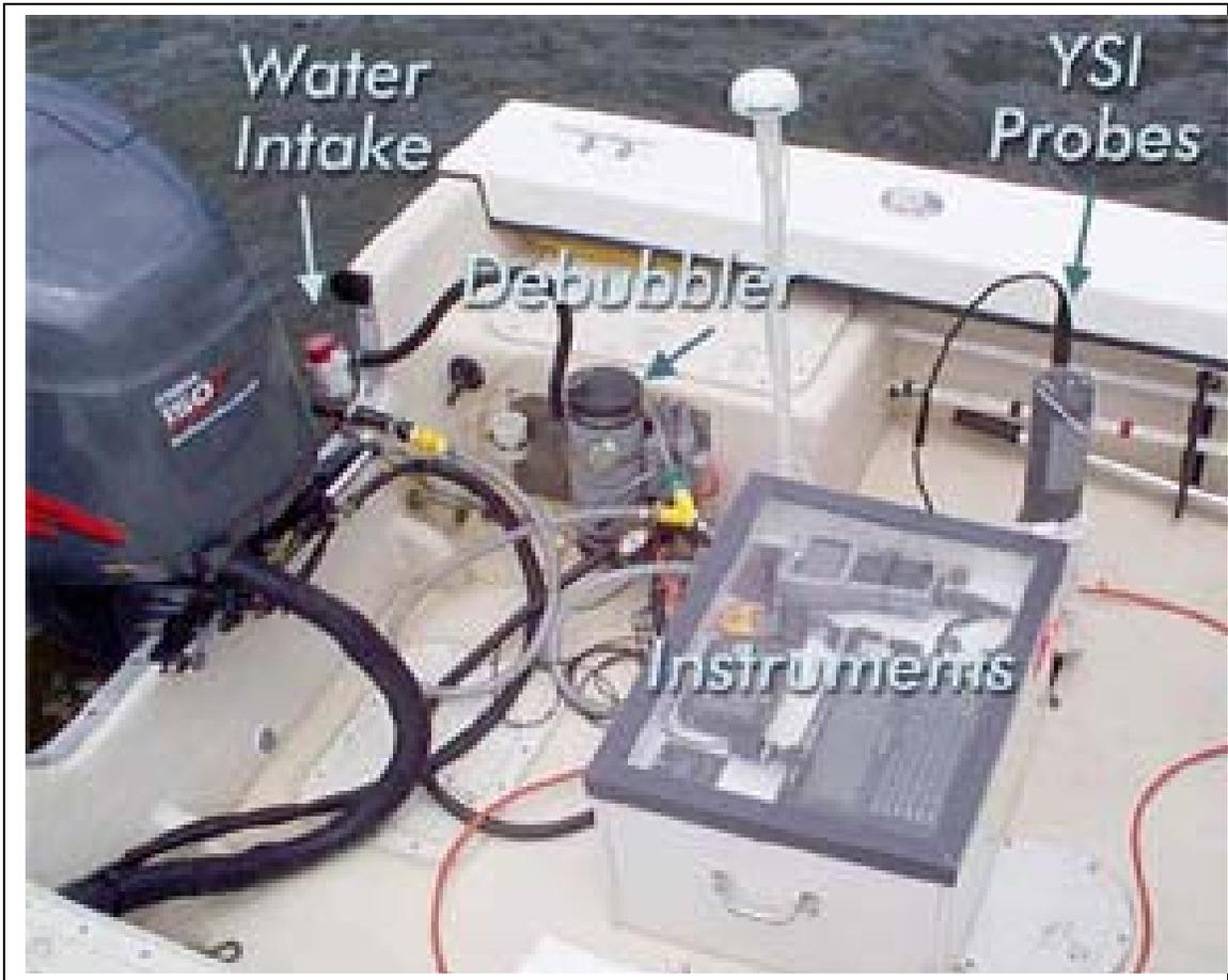
Figure 1. The flow-through DATAFLOW system (*Maryland Department of Natural Resources*; [http://mddnr.chesapeakebay.net/sim/dataflow\\_instrumentation.cfm](http://mddnr.chesapeakebay.net/sim/dataflow_instrumentation.cfm))
