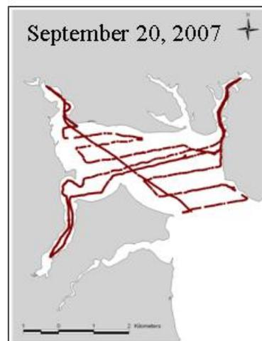
Figure 2: DATAFLOW cruise tracks on the five completed surveys in Greenwich Bay.
