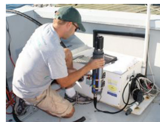
Setting up the DATAFLOW water quality mapping unit.
